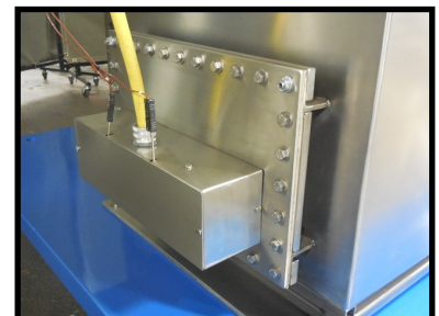
Heating Elements Mounted in Clean-Out Door
