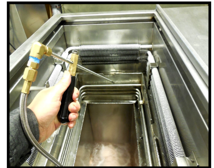
Hand Operated Spray Lance System
