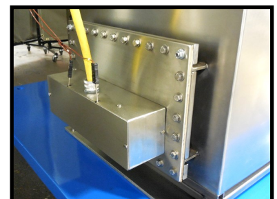
Heating Elements Mounted on Clean-Out Door
