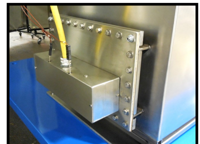
Heating Elements Mounted on Clean-Out Door
