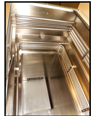
Sub-Zero Coils Operating at -20F for enhanced containment
