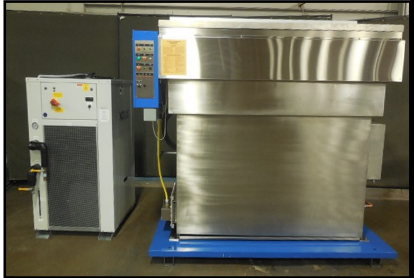
ULTRA VS with chiller
