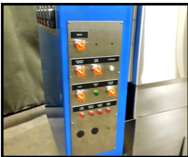
Simple Control Safety Panel
