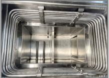
Sizable Ultrasonic Sump (9"L x11"W) with Full Access to Boil Sump
