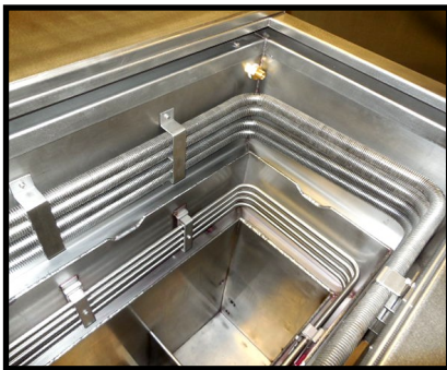
Primary & Sub-Zero Coils running standard refrigerant
