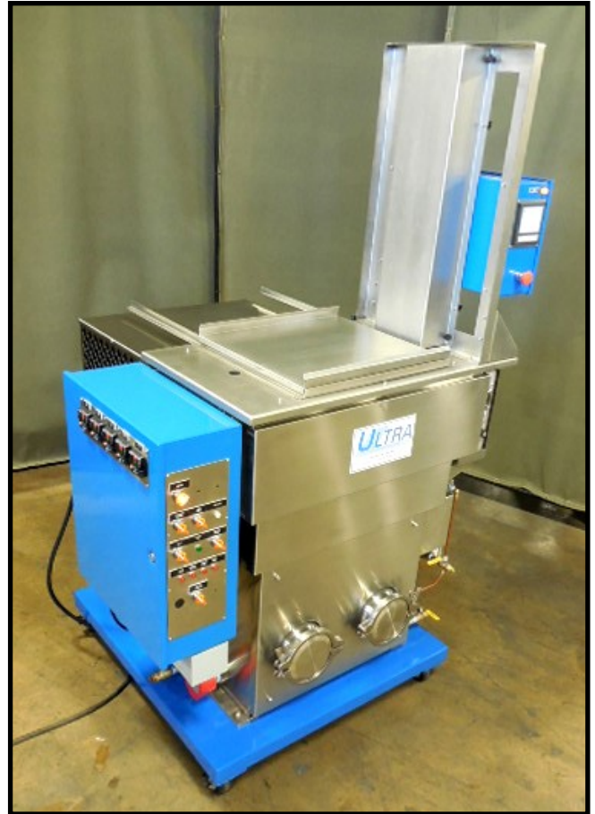
Optional Vertical Basket Handling System for loads up to 25 lbs.
