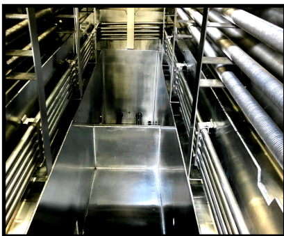
Primary & Sub-Zero Coils running standard refrigerant
