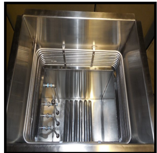
Primary Refrigeration Coils
